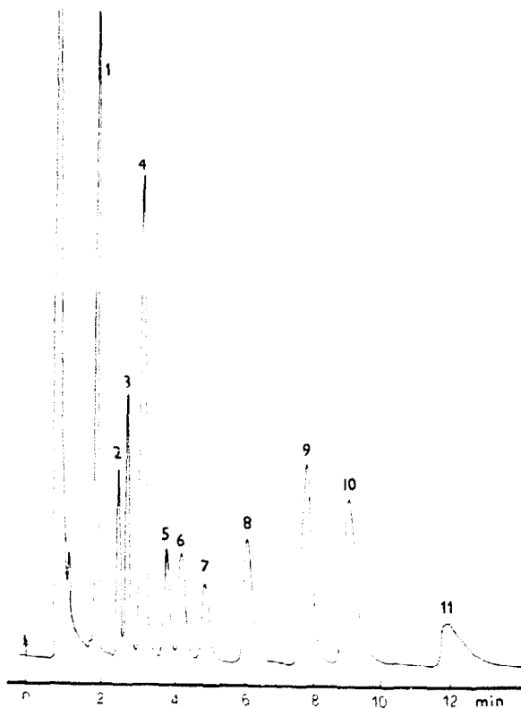
Fig. 5. Separation of phenols: (1) 2,4,6-tri- tert -butylphenol; (2) 2,4,6-trimethylphenol; (3) phenol; (4) 2,4-xyleneol; (5) 2,3-xyleneol; (6) 3,5-xyleneol; (7) 3,4-xyleneol; (8) 2,6-xyleneol; (9) 3,4,5-trimethylphenol; (10) p -methoxyphenol; (11) p -chlorophenol. Stainless-steel column, 500 cm long, I.D. 0.5 cm; glass beads sieve fraction, 50-60 mesh; coating: 0.10% FFAP; carrier gas, nitrogen with p = 0.95 \text{ kg cm}^{-2} and flow-rate 60 ml/min; temperature, 182°.
